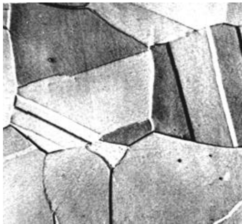
Fig.6.2. Austenite (gamma iron) crystal structure
