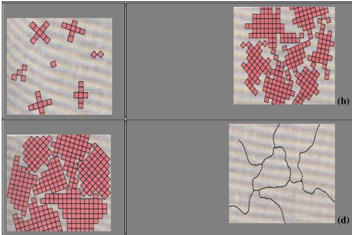
Fig.3.3. Stages of solidification (square grids represent the unit cells).
